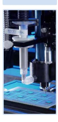
Commonly, customers will purchase two-component epoxies premixed and frozen in syringes for automated dispensing. This removes the weighing step and ensures that material has already been properly mixed for two-component systems.
